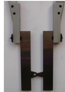
Zeroing for external pitch diameter measurement without the use of a calibration plate.
