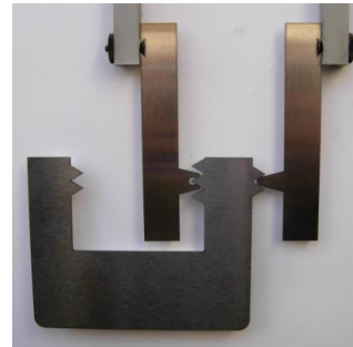
Checking/ calibrating external pitch diameter measurement with the use of a calibration plate.
