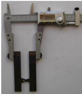
Zeroing for external pitch diameter measurement without the use of a calibration plate.
