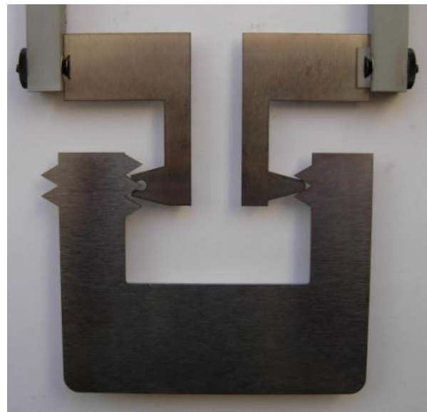
Zeroing for internal pitch diameter measurement using a calibration plate.
