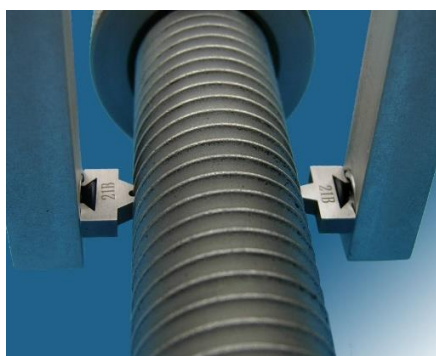
d2 (external pitch diameter)
